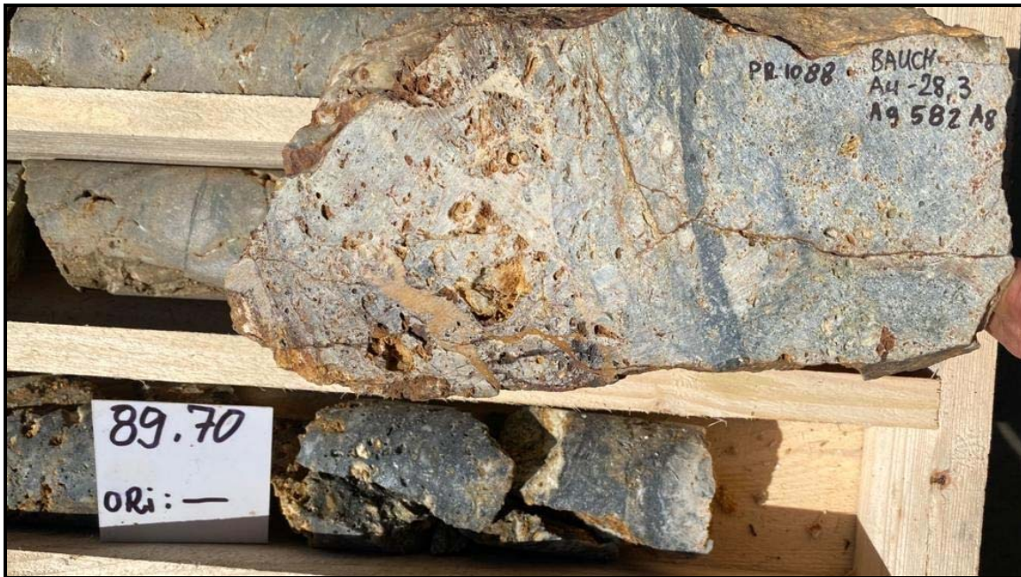
Comparison of the mineralisation style from high grade in situ underground sample (PR1088, 28.3 g/t Au and 582 g/t Ag) and drill core in BADD001. This 0.5m section of the core assayed 17.2 g/t Au and 494 g/t Ag)
