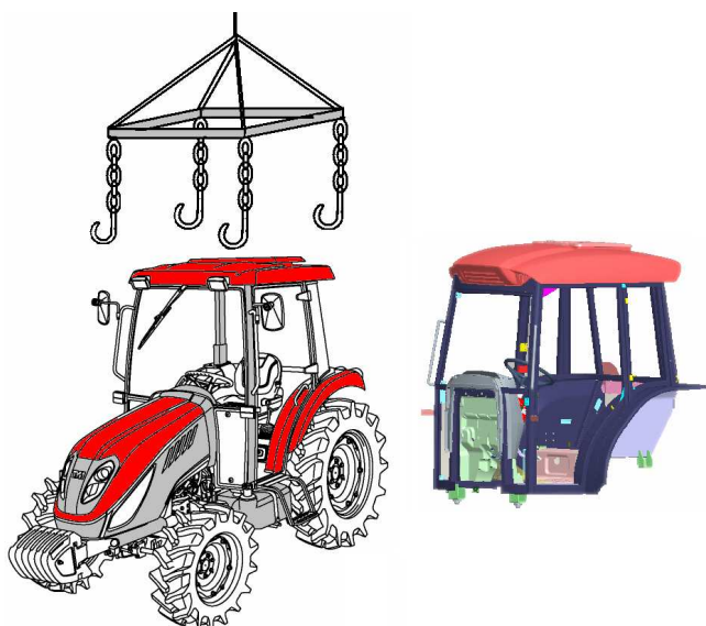
Fig.11-3 Remove the Cabin assembly.
