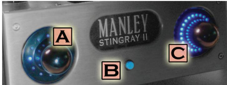
**A) Input Selection & Menu Control:** This knob displays and allows the selection of any one of the 4 inputs available on your Stingray II. The LEDs show which input is selected, starting at the 9:00 position for Input 1 and ending at the 12:00 position for Input 4 (1/8" input). It also allows access to the Menu functions of the Stingray II, including individual input gain adjustment and remote control modes. For more information on these functions, see page 9.
