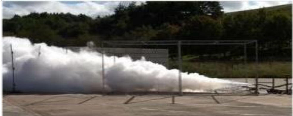
Controlled LH2 release profiled by NREL's HYWAM point-based sensor apparatus
