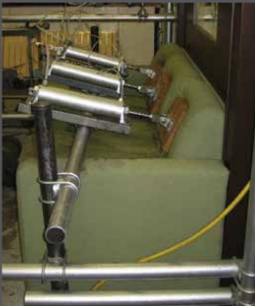
Backrest Frame Test (#7.2.3.2); 150lbs
