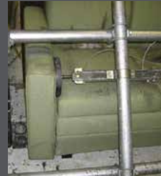
Sidethrust Load on Arms Test (#7.3); 150lbs
