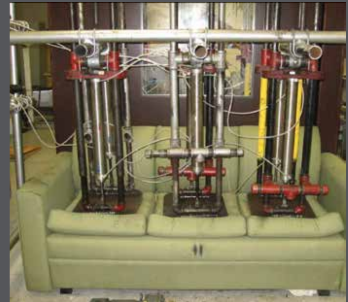
Seat Load Test (#7.1); 275lbs @ Back, 137.5 lbs. at Front
