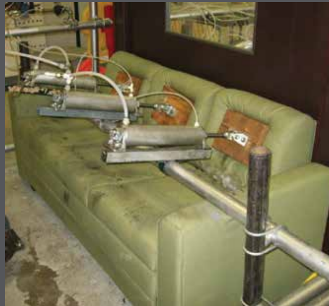
Backrest Foundation Test (#7.2.3.1); 150lbs
