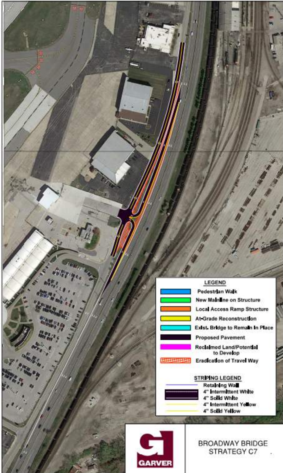
Figure 4: Strategy C7 – Right-In/Right-Out At-Grade Access Improvements
