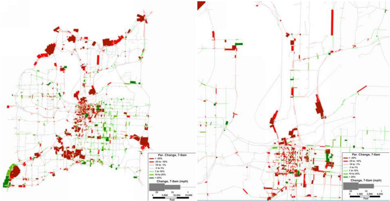
Figure 5-4: A.M. No-Build 2016 vs. 2040 Speed Maps
