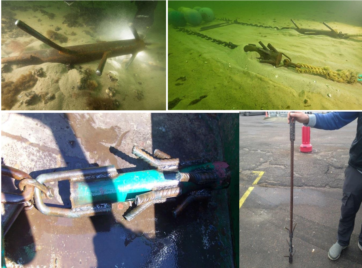
Figure 16 Upper right and left: different search devices used by the German MARELITT Baltic partners, designed by Polish fishermen prior to the initiation of the MARLITT Baltic project. The pictures show two different lengths of the rods, long rod (upper left) and short rod (upper right), ©Christian Howe. Lower left: creeper used in Poland © WWF Poland, Lower right: MARELITT Baltic Estonian creeper used on hard and mixed bottoms ©KEST.
