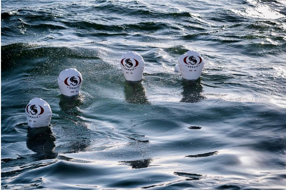
Figure 14 Picture of airbags that are used to lift up the net to the surface when parts or the whole ALDFG is disconnected from the wreck ©Keep Sweden Tidy.
