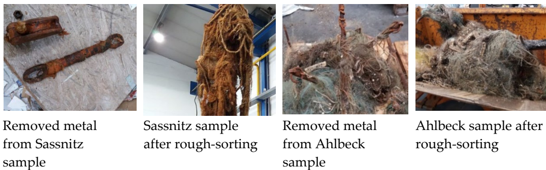
Fig. 2.16: Material outputs from rough-sorting, © F. Schneider
