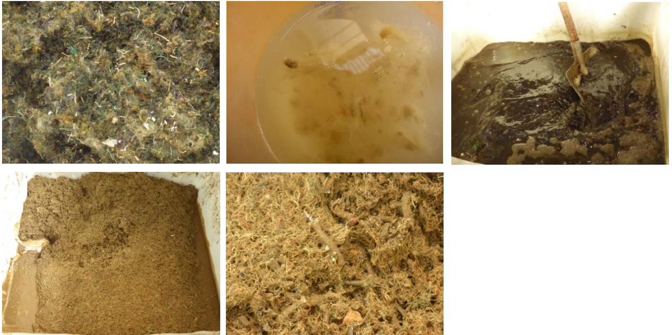
Fig. 3.3: Top panels: The fluffiness of the fibre material impedes complete density separation of the mixed materials. Residual sediments cause the saline solution to become dirty, affecting the density. Bottom panels: Bottom sediment contains silt and fibres entangled with other materials, including sheathed lead lines (middle of lower right panel).
