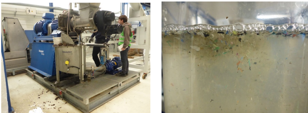
Fig. 3.4: Left: Friction cleaning unit with pump and pipe on the lower-middle right. The catching tank flowed over as the pump filter became blocked by the fine fibres. Right: Small coloured and black particles can be microplastics included in the fishing nets, but might also originate from scrubbing and previous cleaning runs in the friction cleaning unit.
