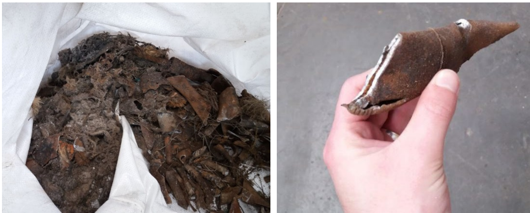
Fig. 2.17: Metal fragments collected by the magnetic separator after rough-shredding, © F. Schneider
