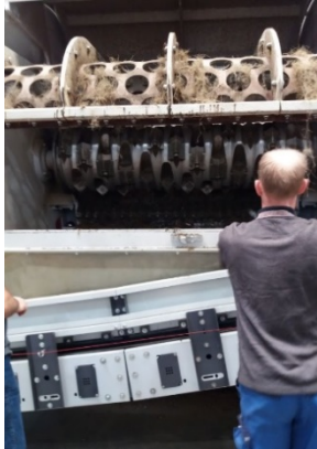
120mm diameter sieve and U-rotor of VAZ 2000 MNFT used for rough-shredding
