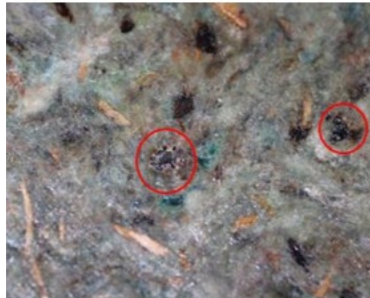
Fig. 6.13: Left: Plates were pressed from gillnet fibre material in different grinding qualities. Right: The microscopic image of the input material reveals a rubber fragment among the inhomogeneous fibre mix. (© Weißbach & Gerke 2018)
