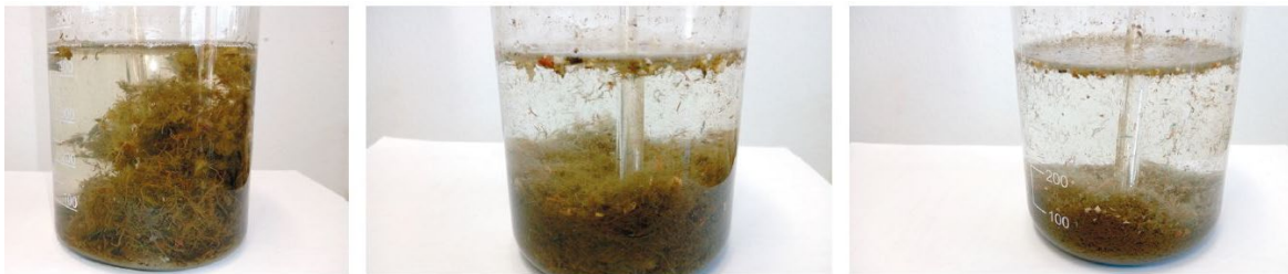
Fig. 6.9: Density separation trials with raw input material a) 20mm shredded, b) fine-ground to 1mm grain size, c) fine-ground to less than 0.5mm grain size. (© Weißbach & Gerke 2018)
