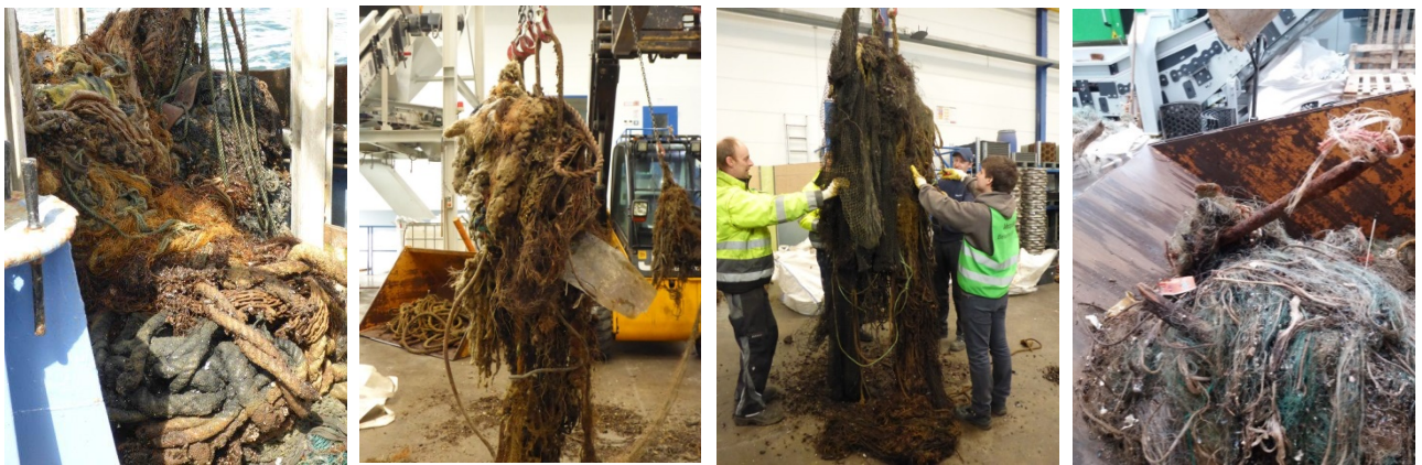
Fig. 1.2: Retrieved lost fishing gear is comprised of a mix of ropes, nets, lines and other materials. Large metal items such as anchors need to be removed to protect machines from damage.
