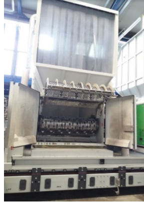
VAZ 1600 M XL T with 20-30mm diameter sieve and a U-rotor for fine-shredding
