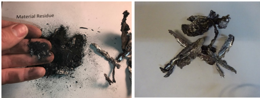
Fig. 5.4: Solid residue: magnetic dust with iron content (left) and recondensed lead fragments (right). © EXOY
