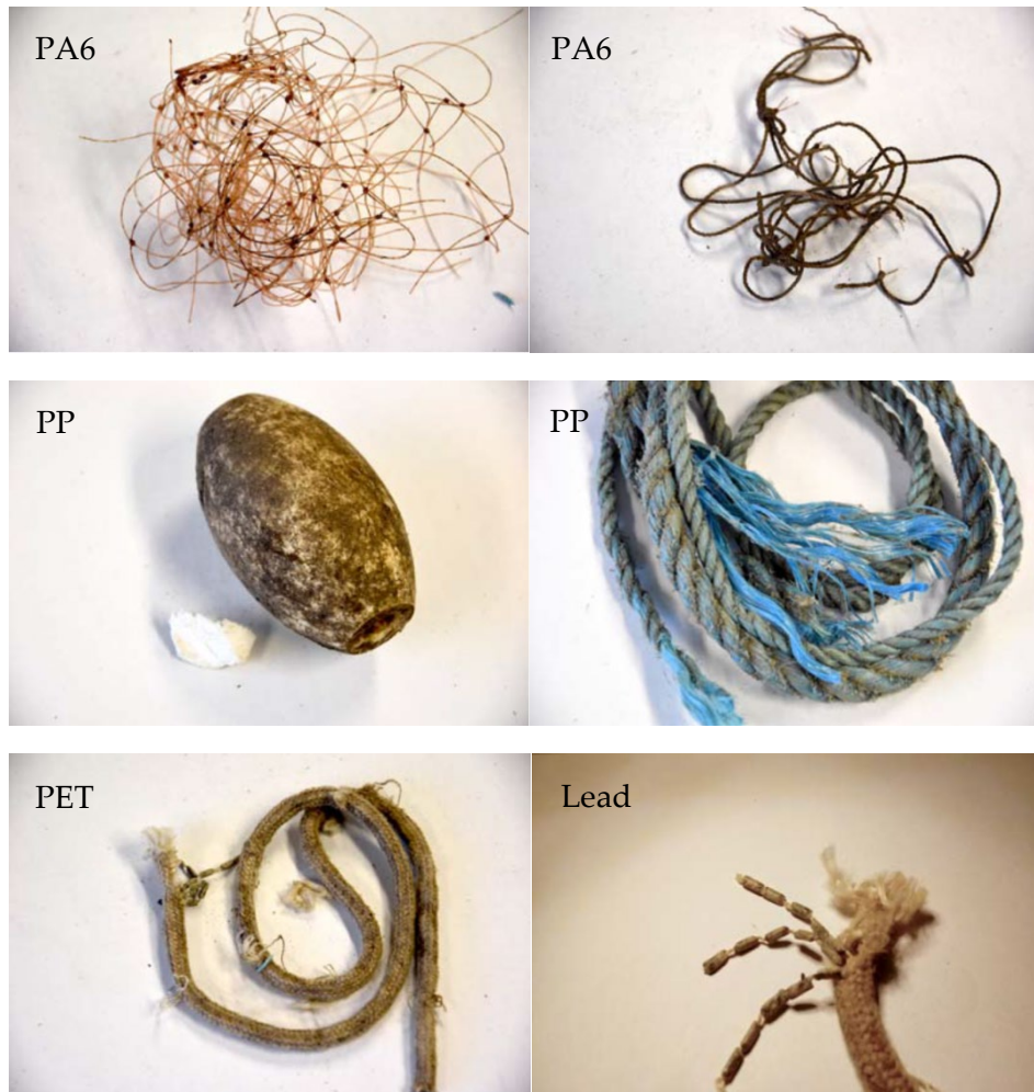
Fig. 6.1: Sample materials from Ahlbeck gillnets. a) Monofilament line, b) twisted line, c) float, d) rope or swim line, e) sink line sheathing, f) lead fragments embedded in sink line. © Gerke & Weißbach 2018
