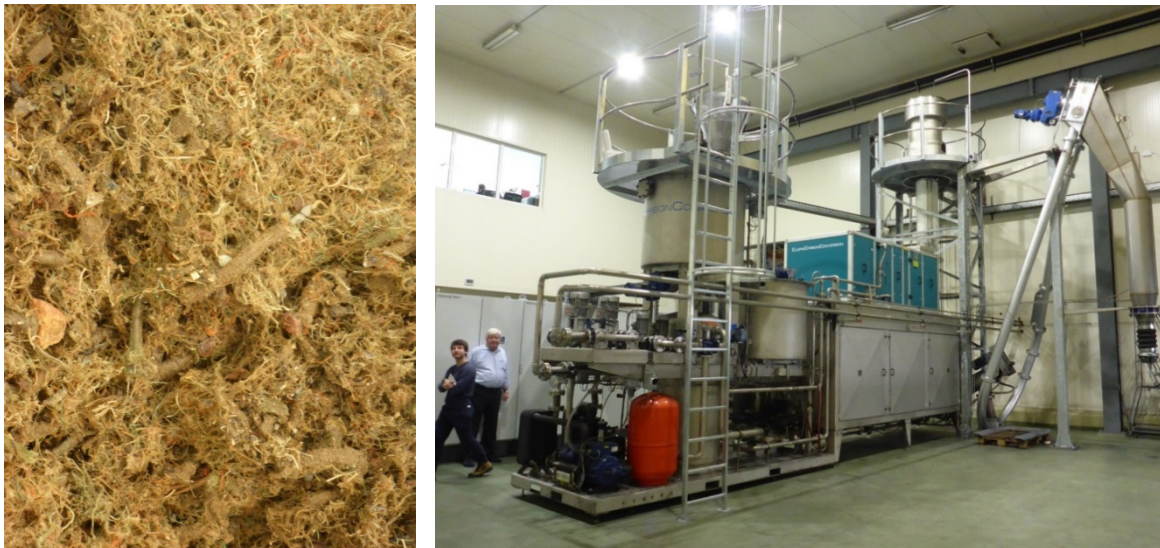
Fig. 5.3: Gillnet feed material used for thermal processing (left). UHTH processing reactor at EXOY's waste recycling facility in Freienbach, Switzerland (right).
