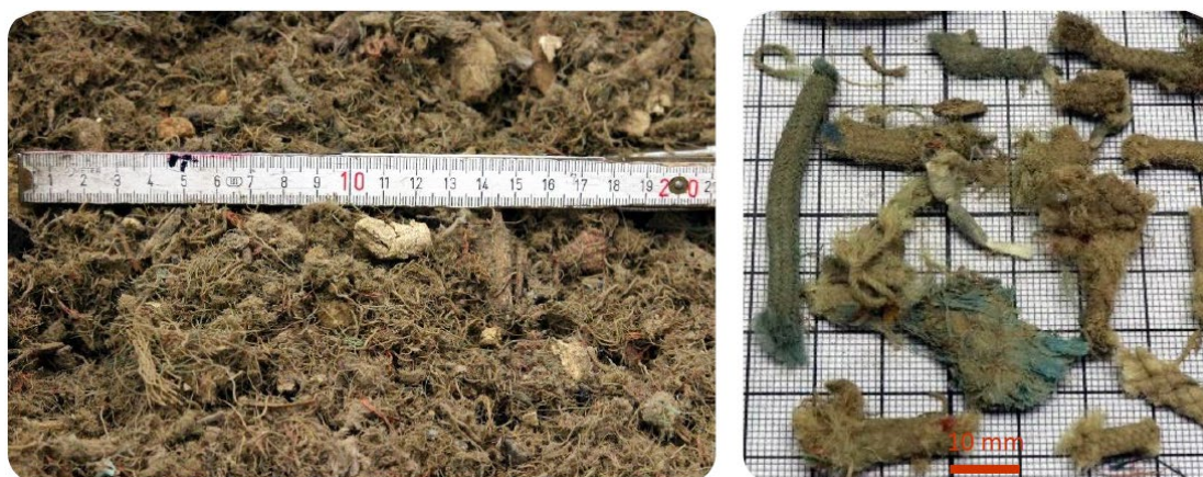
Fig. 5.6: Gillnet-dominated input material (left) and sink line fragments composed of mantled lead (right). © TEER\RWTH Thomas Horst, Johann Hee
