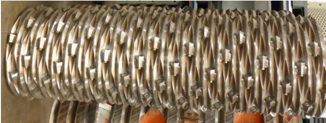
Fig. 3.2: The rotator drags the material into the cutting unit and the triangles form the counterblades to the cutting knives. Triangles are fixed with bolts for easy replacement, and will be expelled if large metal items or rocks are encountered. Without pre-sorting, damage to counter-triangles and cutting blades would require frequent and expensive replacements.
