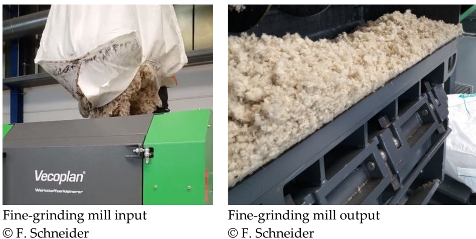
Fig. 2.12: In- and output of the fine-grinding mill
