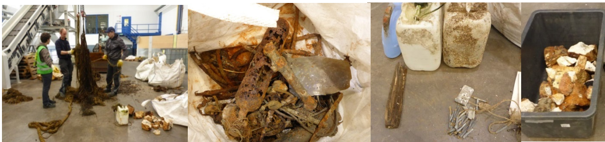
Fig. 3.1: Manual pre-sorting of DFG lifted with a crane to facilitate access. Metal items, canisters, and rocks were manually removed to avoid machine damage during shredding.
