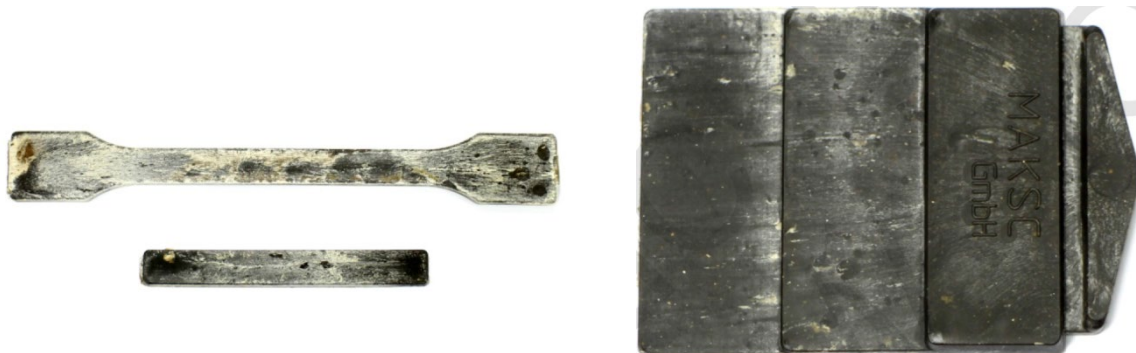
Fig. 4.7: Test specimen of Ahlbeck gillnet sample for mechanical strain tests (© MAKSC GmbH).
