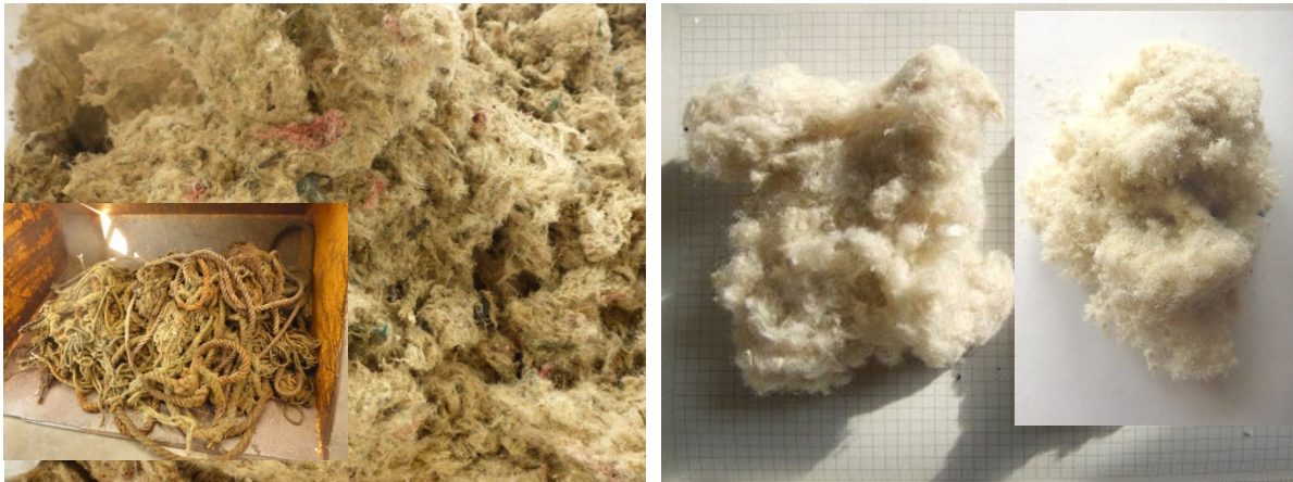
Fig. 4.3: Fibres extracted from ropes before (left) and after friction cleaning (right), shredded and passed through a 20mm sieve (right image, left sample) and the same fibres fine-ground to a grain size of 4mm (right image, right sample) in order to achieve pourability for extrusion and regranulation.
