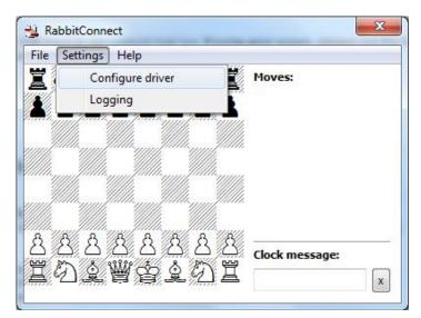
After a few seconds (up to 10) the big square box should turn green and show %Board alive+. Depending if you have a DGT3000 or DGT XL clock connected and switched on, the second box will also turn green and a clock version will be visible.
