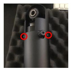
**Step 14:** Unscrew the cap where the airline goes to the shock.
