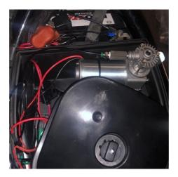
**Step 5:** Place the compressor so that it does not interfere with the air filter or air box cover when closed. Drill two ¼ inch holes like shown below and in the diagram on the last page. Use zip ties to hold down the compressor.
