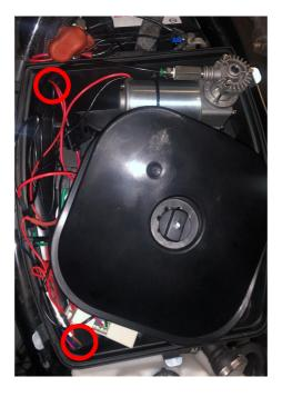
**Step 7:** Place the relay, fuse, and remote-control relay, and the compressor into the air box. Use the wire diagram on the last page to connect the electrical wires of these four components.
