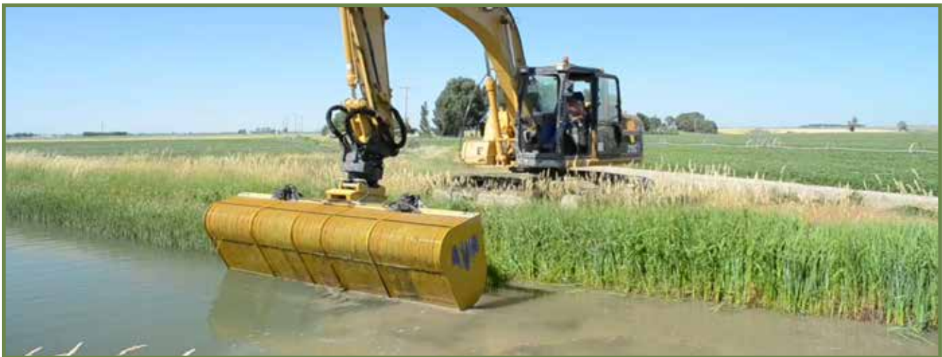
Figure 14. Mechanical control using the aquatic vegetation rake (AVR) on irrigation canals near the Snake River (Photo credit: Aberdeen-Springfield Canal Company)
