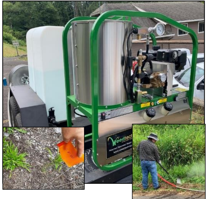
Figure 2 clockwise, starting at the top: 1) Trailer mounted steam machine, 2) steaming vegetation along a roadside, 3) regrowth of oxeye daisy two months post-treatment.
