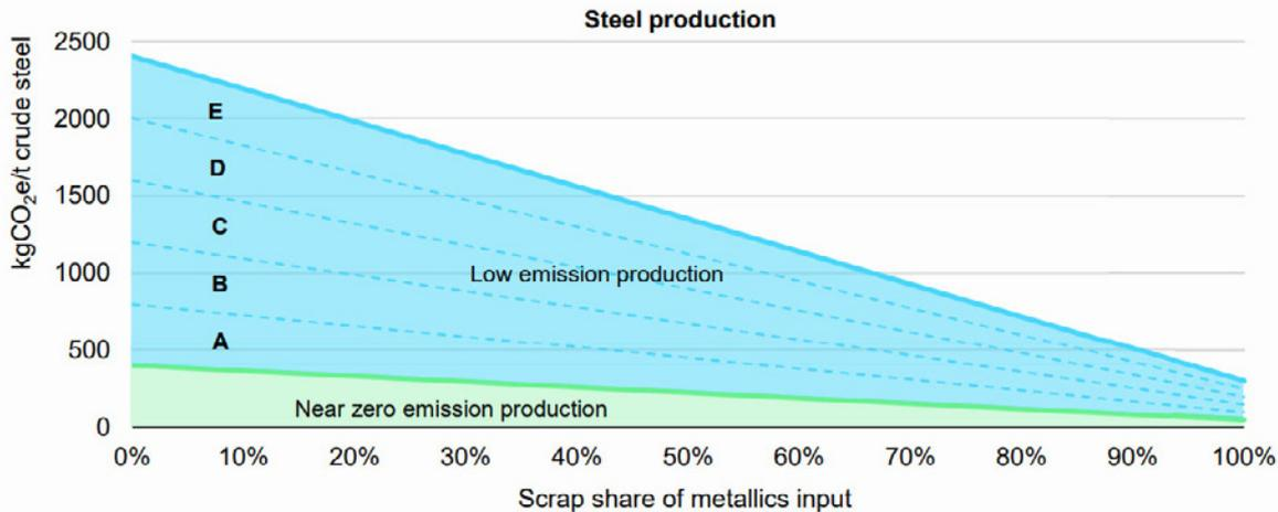
Figure 1: IEA’s near zero emission crude steel production threshold as a function of scrap use and proposed classification system (Levi et al., 2022).
