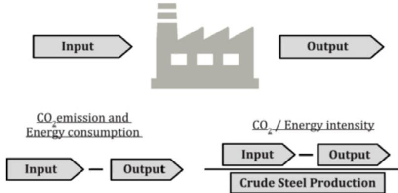
Figure 10: Conceptual framework for the calculation of emissions from steel production in ISO 14404-4:2020 (ISO, 2020) .
