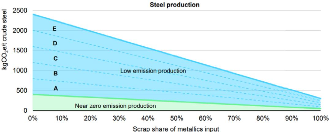
Figure 13: IEA’s near zero emission crude steel production threshold as a function of scrap use and proposed classification system (IDDI, 2022a).
