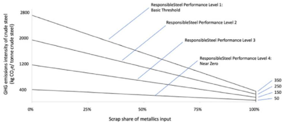
Figure 3: ResponsibleSteel’s Performance Level breakdown for crude steel emissions intensity including a sliding-scrap utilization scale (ResponsibleSteel Standards and Certification, 2022).
