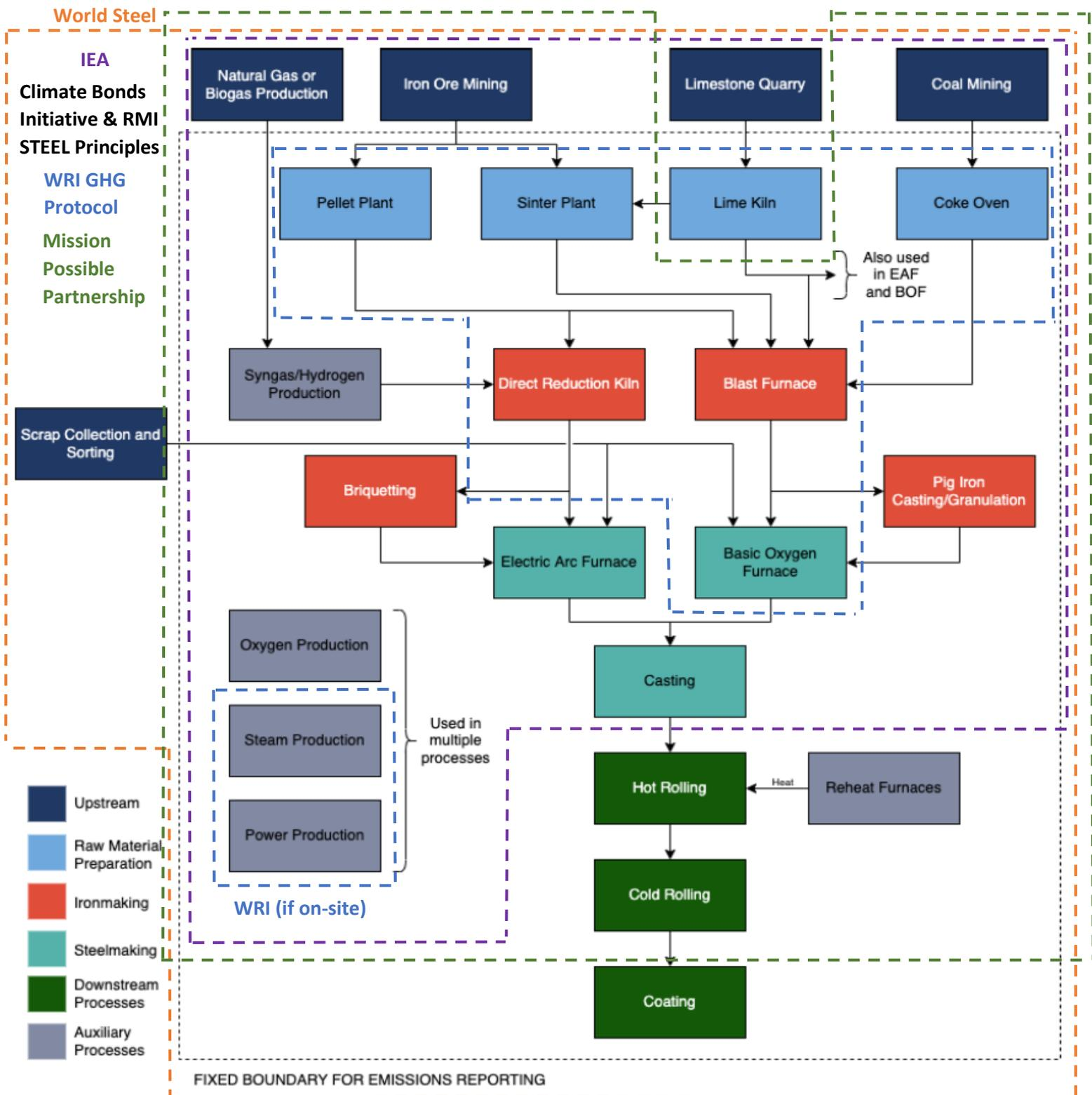
**Figure 2:** Comparison of system boundary of several steel decarbonization standards, protocols, and initiatives. (It should be noted that around 90% of CO<sub>2</sub> emissions in primary steelmaking is related to ironmaking processes (blast furnace, sintering, coking), which are included in all system boundary shown in the figure.)
