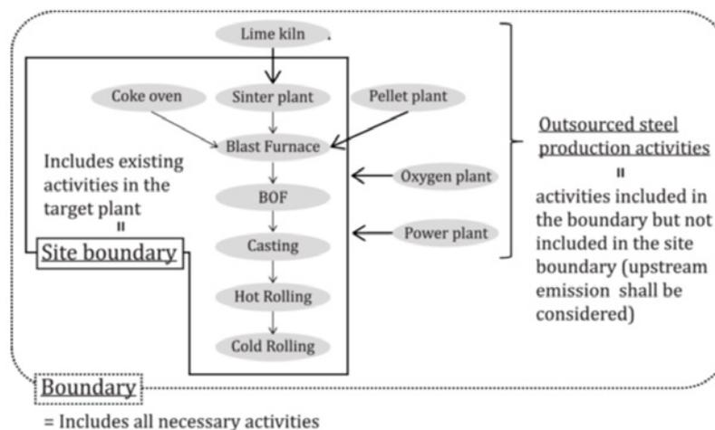
Figure 11: ISO 14404 diagram of emissions boundary and site boundary (ISO, 2020).
