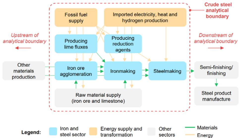
Notes: "Other materials production" refers to the production of material inputs to the iron and steel sector besides iron ore and limestone, including electrodes, alloying elements and refractory linings. IEA. All rights reserved.
