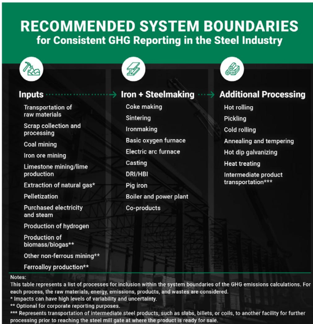
Figure 12: AISI’s recommend system boundaries for GHG reporting in the steel industry (AISI, 2022d).
