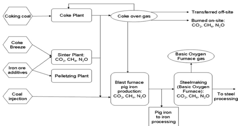
Figure 4: The main GHG emissions sources associated with iron and steel production included in the WRI GHG Protocol for Steel (Russell, 2008).
