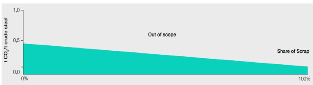
Figure 18: The First Movers Coalition's scrap proportional sliding scale required to meet the definition of near-zero emissions steel (First Movers Coalition, n.d.).
