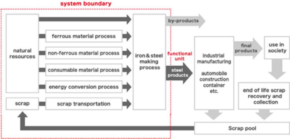
Figure 32 System boundary under JIS Q 20615 (The Japan Iron and Steel Federation, n.d.).
