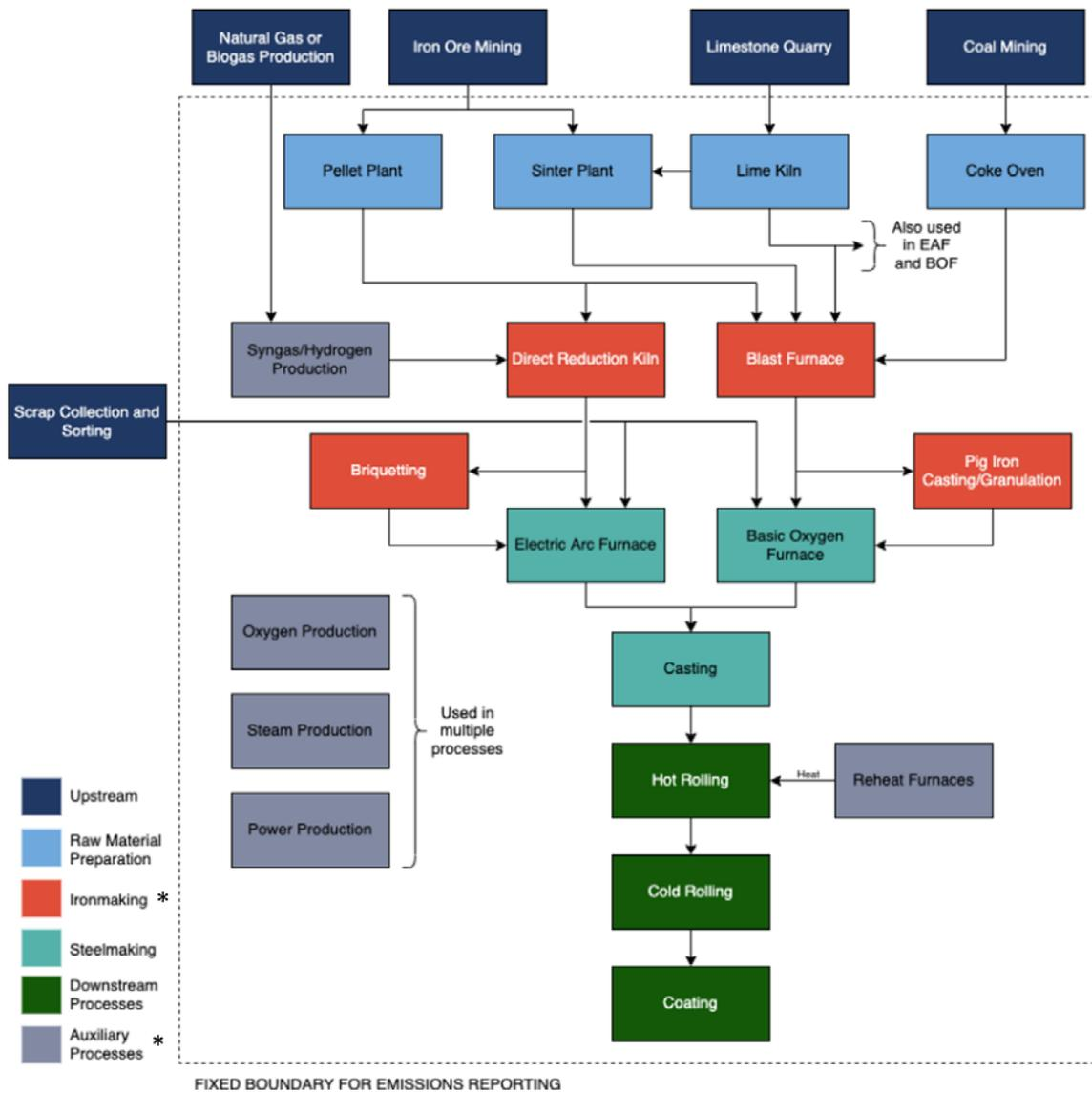
Figure 19: Fixed System Boundary of the RMI’s Sustainable STEEL Principles (Sustainable Steel Principles, 2022b).
