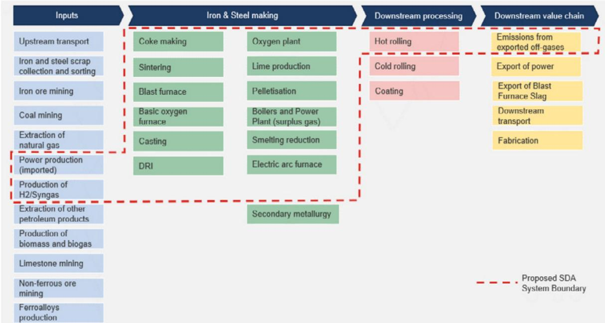
Figure 16: Iron and steel industry core SDA boundary proposed on the draft 1.5°C Steel Science-Based Target Setting Guidance.
