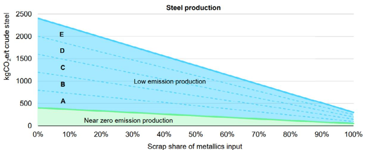
Figure 27: IEA's near zero emission crude steel production threshold as a function of scrap use and proposed classification system (Levi et al., 2022).
