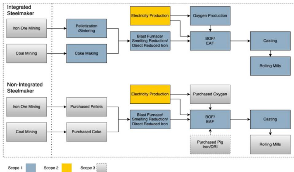
Figure 20: Example of Scope 1, 2, and 3 emissions within the Fixed System Boundary for the RMI’s Sustainable STEEL Principles (Sustainable Steel Principles, 2022b).
