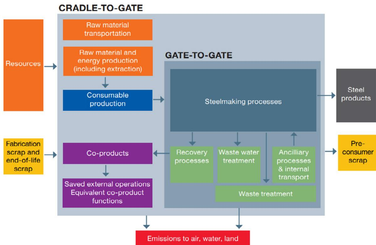
Figure 8: LCI Boundary for steel produced without scrap from the World Steel Association’s LCI Methodology Report 2017 (World Steel Association, 2017).
