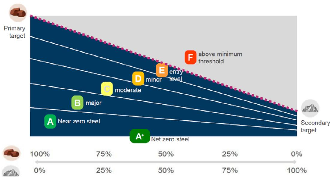
Figure 23: ArcelorMittal proposed Low-Carbon Emissions Steel Standard scoring system considering steel emissions intensity and scrap utilization (ArcelorMittal, 2022b) .
