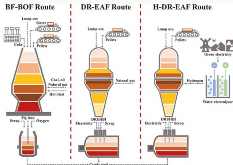
Figure 1. The production process for BF-BOF, natural gas DRI-EAF, and H<sub>2</sub>-DRI-EAF (Wang et al. 2021)
