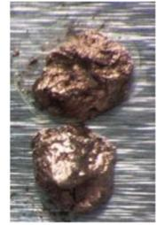
Fused nanocopper, 300 micron size dots
