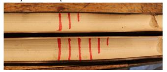
culm on the pith side using Sharpie indelible markers- for a two piece rod, I use BLACK to mark the Butt section, and RED to mark the Tip section. If I'm making a 3- or 4-piece rod, I will use other colors to distinguish the appropriate mid-sections. The two sections of
