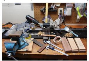
blades, Japanese Dozuki saw, files, scrapers, dial calipers (with and without a Waara V-block attachment for strip measurement), dial depth indicator, center gauge, files and adjustable steel planning form. Although some makers still use planning forms for primary and secondary treatment of bamboo splines, I complete these steps with my bench-top rough beveller (Bellinger Inc., see Step 9 below).
