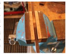
There are various node-spacing protocols, but I usually tend to use 3 by 3 spacing pattern. After node displacement, I use my Dozuki saw to cut the Butt and Tip strips to their proper length (which varies for each rod). The smooth protrusions that remain after careful
