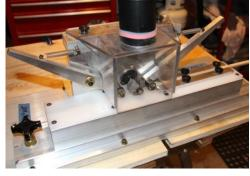
tip strips are  $\sim$ 0.2". The rough beveller speeds up the process of initial strip preparation- it takes about 1 h to machine taper all of the strips, compared to  $\sim$ 12-15 h using a hand-plane and a set of rough wooden bevelling forms.
