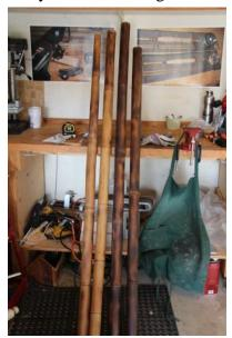
toned, while the other has been flamed to a medium brown tone. Even though there are some slight differences in the surface hue, the underlying cane itself is surprisingly consistent in tone. A definite advantage of flame toning is that the color of the final rod can be enriched, producing beautiful hues ranging from carmel to dark brown. By driving out excess moisture, the stiffness of the cane rod can also be increased, enhancing its action.
