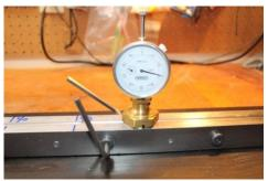
depth of the form can be adjusted at 5 inch intervals by tightening or loosening bolts that draw together or push apart the two sides of the form. This adjustment along the form is what determines how the individual bamboo strips
