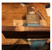
These must be smoothed by filing to facilitate the next steps of splitting. I use a single cut flat-mill bastard file to carefully remove the nodal ridge
