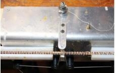
After final planing is completed, the rod sections are glued and bound. After 3-4 days of curing, the rod sections are cleaned and buffed. This process culminates in the generation of a fine set of blanks- one butt section and two identical tip sections.
