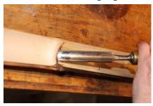
rubber mallet to remove the pith from the inner portion of each node as shown in the figure on the left. After removing the pith, the inner nodal section is nearly even
