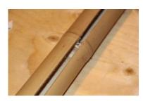
Broker). Typically, the rod maker introduces a "check split" into each culm to allow for expansion and contraction, which reduces the likelihood of producing cracks elsewhere in the culm during storage.
