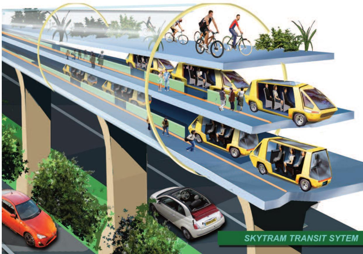
The above sketch is one possible configuration of the support and upper superstructure for the Skytram system. The column support could be a single column underneath, one column on each side or a combination depending on the surface it is going over. Again, the general description is that of an advanced, or expanded, 2 or 3 story skyway, like the existing skyway system.
