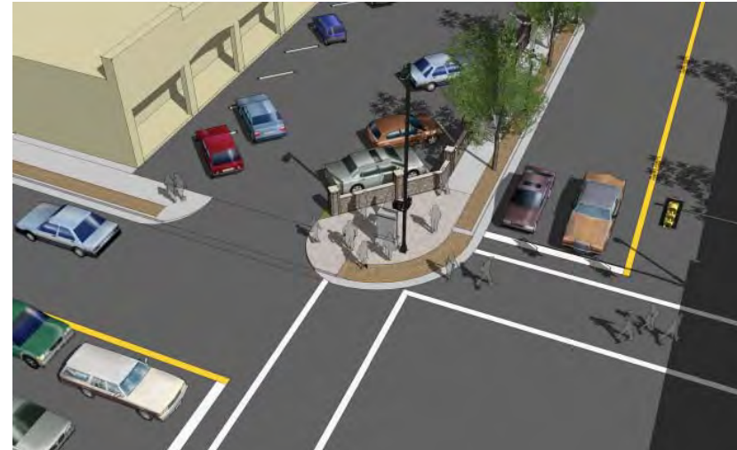
Figure I – Kensington & 10 St NW Pedestrian Refuge AFTER
