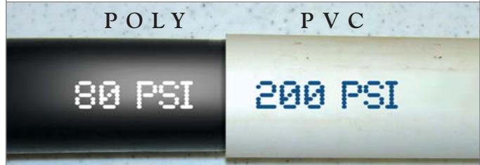
The American Society for Testing and Materials (ASTM) has established industry rating standards for pipes. Through stringent testing, they have rated the PVC pipes that DRF uses at 200 PSI and the poly tubing our competitors use at 80 PSI. These ratings are stamped on the pipe, and regardless of the installer's personal preference or belief, it proves that PVC is 2 1/2 times stronger than poly.
