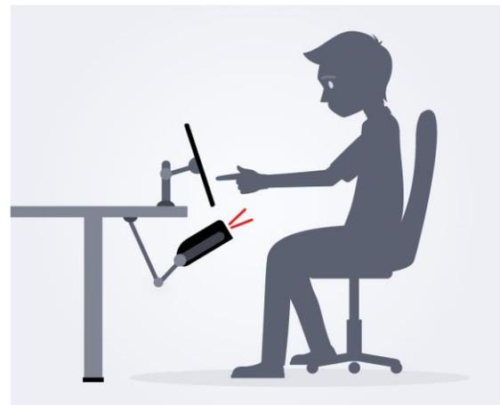
**Figure 5.** Final setup with eye tracker closer to the participant
