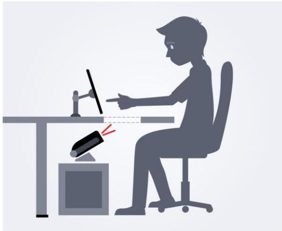
**Figure 3.** Table with a hole and the eye tracker positioned under the table
