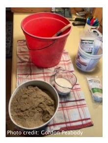
Pictured above: Low tech materials: sand; gelatin; water and mixing container.
