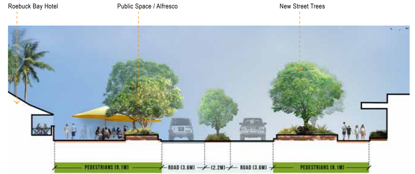
04 Section 04 through Dampier Terrace
