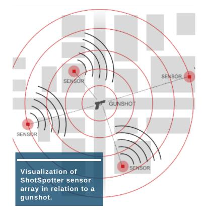
The process begins with SST working with the customer to determine the desired physical boundaries for ShotSpotter's gunshot detection technology. Ultimately, the choice of boundaries is one for the customer, considering the needs and resources of the particular community. The larger the coverage area, the greater the cost.
