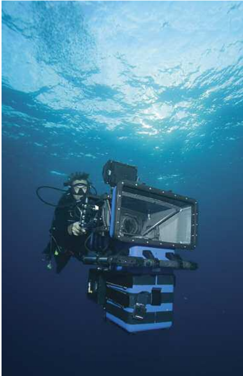
Underwater camera operator Simon Christidis, ACS wields the camera rig, which is safely encased in Cameron-Pace Group's underwater housing.
