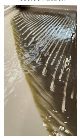
Multi-Gravity Separator -50 micron fraction
