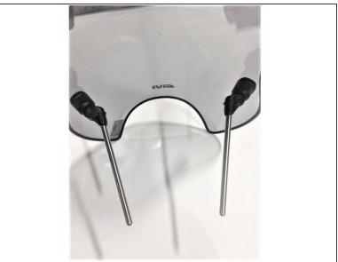
Mount the arms to the windshield hardware previously installed using the supplied hardware.
