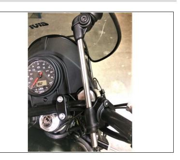
Insert the assembled windshield bars into the clamps, tightening the hardware until snug yet loose enough to adjust the position of the windshield.
