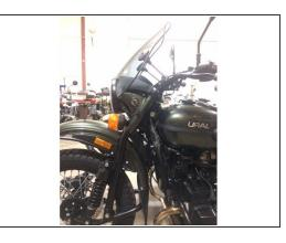
Take a look from the rider's perspective as well as the side and front of the motorcycle. Adjust the windshield as an assembly to be centered on the headlight and to suite your desired angle.
