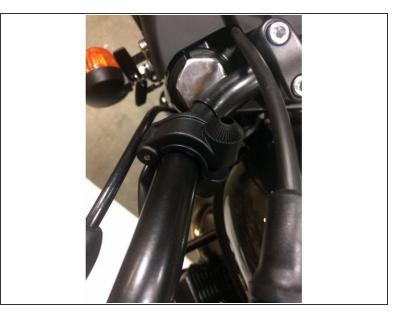
• Fix the clamps onto the handlebars using the supplied spacers. When properly placed they will fit under the wiring of the handlebar without interference.
