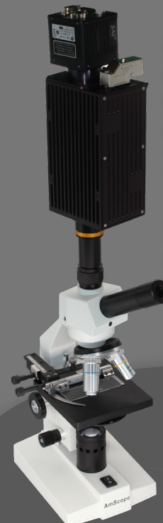
HSI without Integrated PC Compatible with any C-Mount Interface of a Microscope or Telescope
