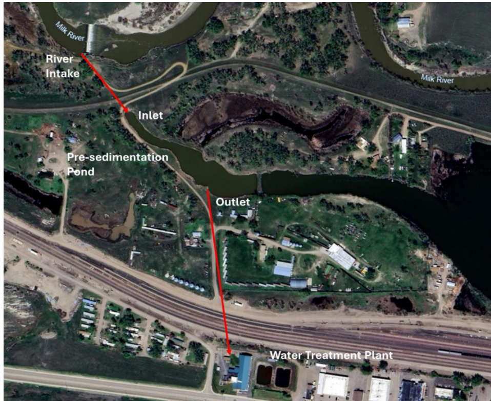
FIGURE 2. Milk River intake, pre-sedimentation pond, and WTP locations.
