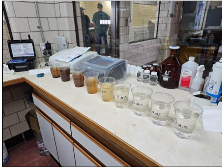
FIGURE 18. Filter No. 1 backwash waste turbidity samples.
