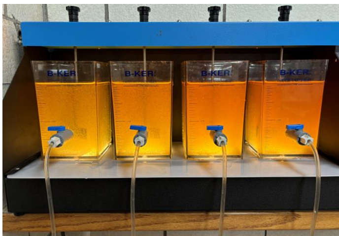
FIGURE 23. Jars during flocculation step showing increasing ferric sulfate dose, left to right.
