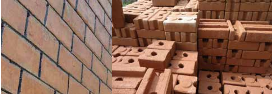
Figure 41. (left) Interlocking Stabilized Soil Blocks. Source. UN-Habitat Figure 42. (right) Interlocking Stabilized Soil Blocks. Source. Sri Lanka Spirit
