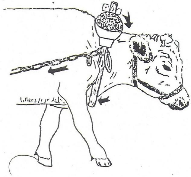
*Fig. 3: Because of the lowered hitch point, the beam of a historical yoke rotates the bows back into the shoulders of the oxen, giving them an additional surface to push against.*
