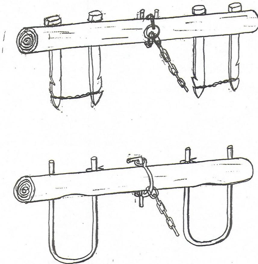
*Fig. 1: Examples of some neck yokes we have seen made from small poles in Africa. The hitch point for the chain is behind the beam. There is little or no carving to fit the neck of the oxen. Rectangular paddles or thin steel bars are used to hold the animals in position.*
