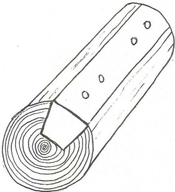
Fig. 9: Traditionally a large tree was split and one section was used to make the yoke beam. This eliminated the heartwood, and the tubular grain
