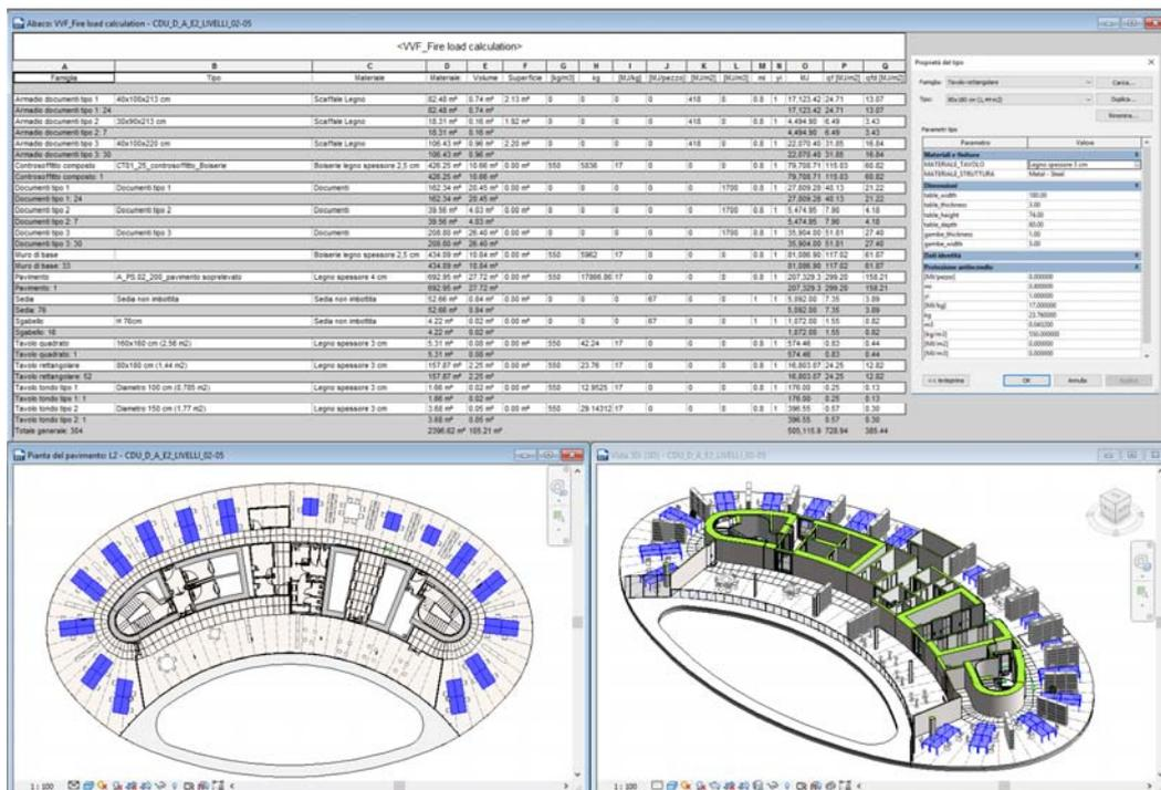
Fig. 4. Fire load calculation
