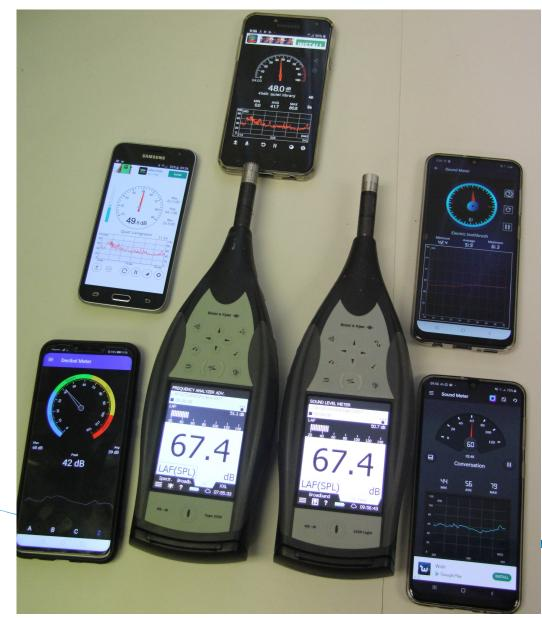
Mobile phone noise meter apps are readily available on line. Unfortunately all the ones we have seen are sadly inaccurate, usually measure the wrong units and seriously mislead users about whether they comply or not.
