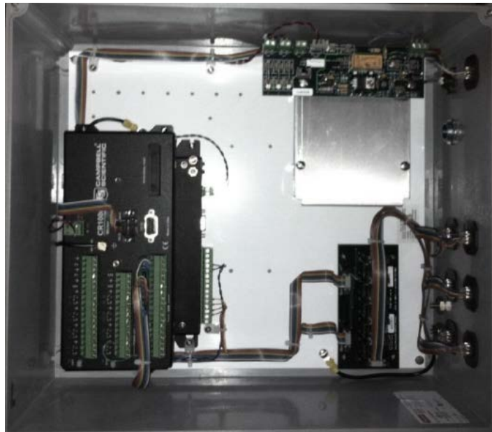
Figure 10. Inside of the Geokon model 8021 Micro-1000 data logger box
