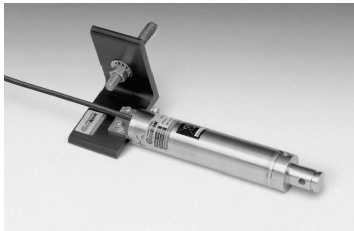
Figure 4. Geokon model 6350 vibrating wire tiltmeter (Geokon Inc., 2013c)
