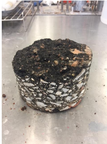
Figure 13. Picture of a Base Core for I-35 SB.
