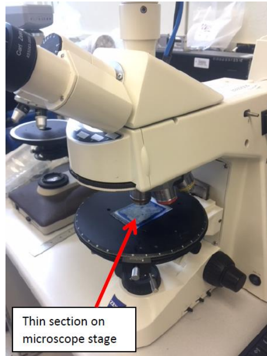
Figure 17. Thin Section Observation under a Transmitted Light Optical Microscope.
