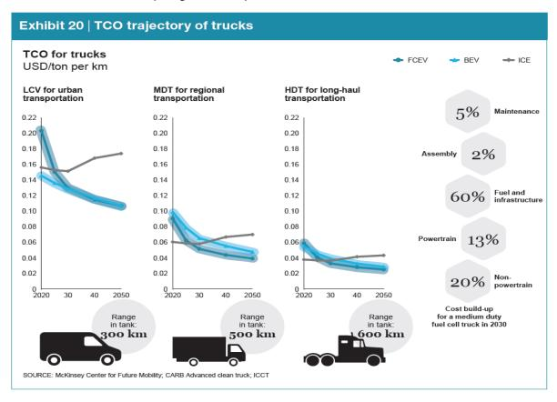
**Fuel cell trucks offer similar operational requirements as conventional vehicles compared to other zero-emission technologies, with a longer range and shorter refuelling time,** however the alternative drivetrain (battery modules, fuel cell and hydrogen tanks) could require some adjustments to the vehicle's architecture. Hydrogen fuel cell trucks have a heavy payload similar to that of combustion engines given the high energy density of hydrogen.
