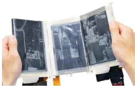
**Figure 2.** PaperFold prototype with 3 display segments.
