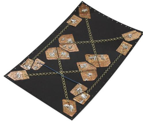
Figure 3. Cardboard actuation layer with Flexinol wires affixed to a copper substrate.
