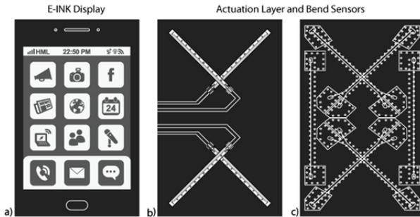
Figure 2. MorePhone layers of flexible cardboard circuitry.
