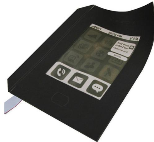
Figure 4. MorePhone displaying shape actuation in the top right corner, with on-screen notification popup.
