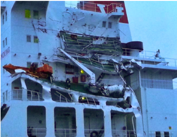
Figure 7: Accommodation damage from bow impact (RNLI)
