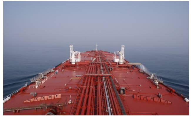
Figure 4: Typical view over fore deck of a double hull tanker, line of double side is about 2.5 m in from ships' sides, beam about 48 m
