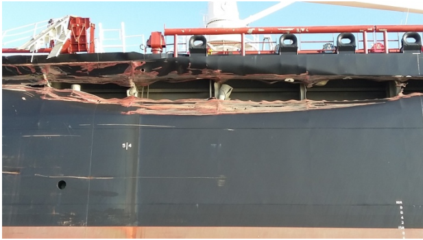
Figure 11: Sideshell damage to moored tanker (allision), note inner hull remains intact
