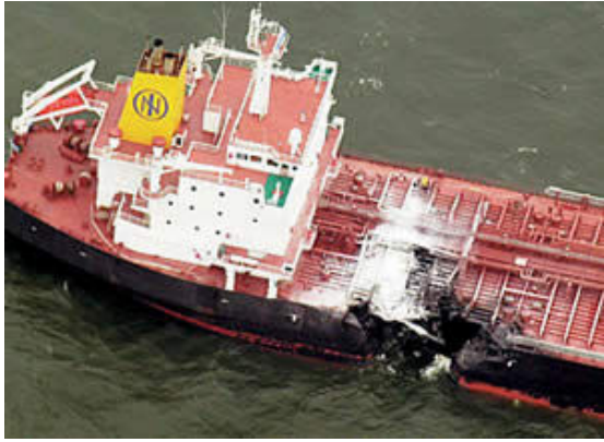
Figure 10: Baltic Carrier after collision, 2001 (photo ITOFF)
