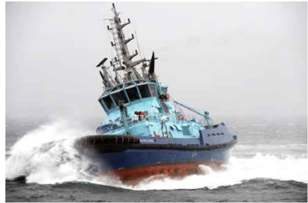
Figure 6: RAstar sponsoned hull form initiated with VSP escort tug – Ajax
