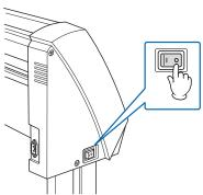
2 Connect one end of the provided power cord to the FC7000 AC line inlet and the other end to an electrical socket of the rated supply voltage. Make sure that the FC7000 is grounded.
