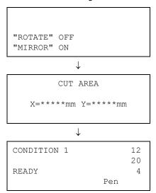
The plotter is now ready to receive data for cutting or plotting. If the interface or command settings have not been made, make these settings before sending the data. If the settings have been made, pen adjustment is performed. When the pen adjustments have been made, the plotter is ready to start cutting. Send the cutting or plotting data from the application software.
