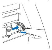
2 Make sure that the bracket of the pen station is engaged in the upper groove of the pen.
