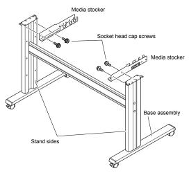
4 Mount the plotter on the stand by inserting the positioning pins on the stand into the positioning holes on the underside of the plotter. Fasten with four socket head cap screws (two on each side), using the Allen wrench. The cutting plotter mounting direction is different for the front loading and the rear loading models.
