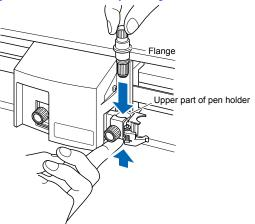
3 Make sure that the pen bracket is engaged on the pen's flange, and then tighten the screw.
