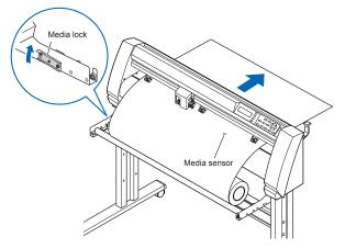
4 Pull the media taut to make sure that there is no slack in the conveyance path, and then raise the media set lever to lower the pinch rollers. Release the media lock.
