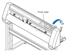
2 Place the media roll on the roll media stocker. Load the media in the plotter as shown. Pass the leading edge o from the back of the plotter so it emerges from the front.
