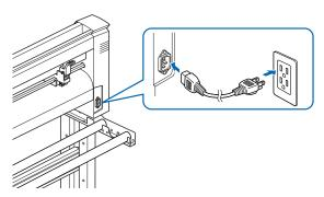
3 Turn on the FC7000 by pressing the "|" side of the switch. The control panel POWER lamp lights.
