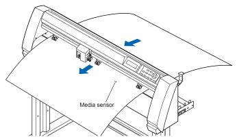
3 Pull the media taut to make sure that there is no slack in the conveyance path, and then raise the media set lever to lower the pinch rollers. If you align the right edge of the sheet with the guides on the platen, the sheet can be loaded so that it is straight.
