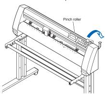
2 Place the media roll on the roll media stocker. Load the media in the plotter as shown. Pass the leading edge from the front of the plotter so it emerges from the back.
