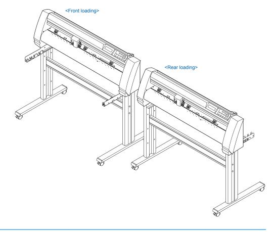
1 Assemble the left and right stand sides. Fasten a base assembly to each of the stand side bars with four socket head cap screws, using the Allen wrench.
