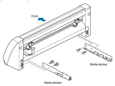
2 Insert an M4 screw in the second hole from the front side of the plotter.
