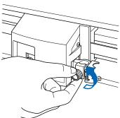
While pushing the pen holder in the upward direction, push the pen all the way into the holder until its flange contacts the upper part of the holder.
