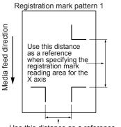
Use this distance as a reference when specifying the registration mark reading area for the Y axis
