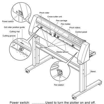
media. The rear sensor is used to sense the trailing edge of the media.
