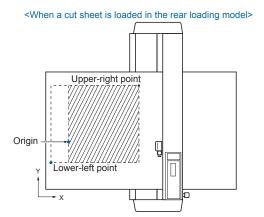
When ROTATE has been selected to rotate the coordinate axes by 90° as shown in the example below, the shaded area represents the effective cutting/ plotting area defined by the LL and UR points.
