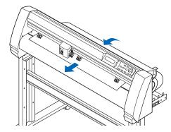
3 Press the media lock to engage it, and then pull the leading edge out of the front of the plotter so that it completely covers the media sensor.
