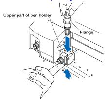
3 Make sure that the pen bracket is engaged on the pen's flange, and then tighten the screw.
