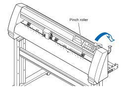
2 Pass the leading edge of the sheet from the rear of the plotter so that it emerges from the front, making sure that is completely covers the media sensor.
