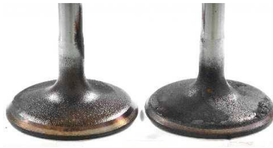
After BG 44K ® 8 mg (94% clean-up) 28 mg (85% clean-up) 9.8 9.2
