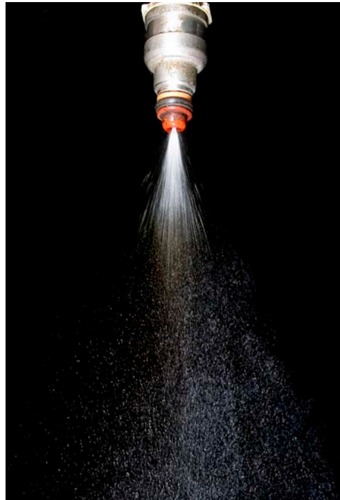
After service with BG Fuel Injection System Cleaner, Part No. 210, the same fuel injector is functioning properly. It mists fuel so that the fuel/air mixture is properly balanced and combustion of fuel is thorough.
