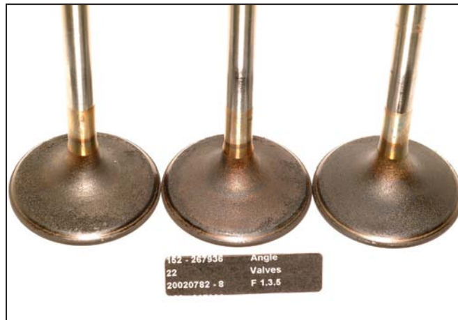
Intake valves after using BG 44K® for 100,000 miles.
