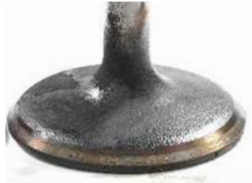
After BG 44K ® IVD Mass: 12 mg (95% clean-up) CRC Rating: 8.9
