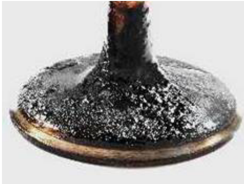
Before IVD Mass: 223 mg CRC Rating: 7.7
