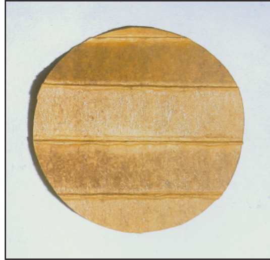
Fuel filter after BG 44K ® .
