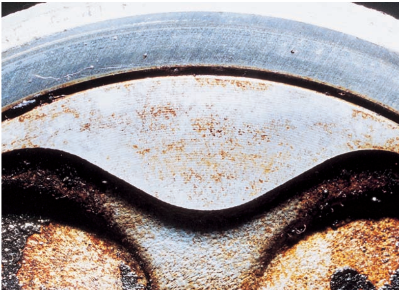
Same combustion chamber squish area after BG 44K ® .
