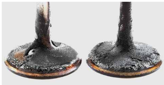
Before IVD Mass: 126 mg 190 mg CRC Rating: 8.0 8.0
