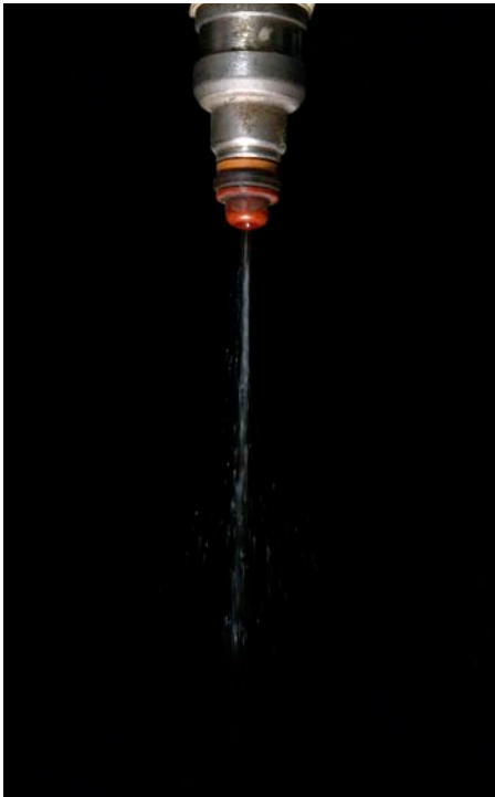
A fouled fuel injector sprays fuel in irregular streams, resulting in improper combustion of fuel and increased exhaust emissions.
