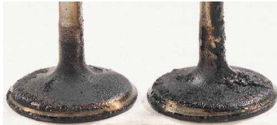
Before IVD Mass: 43 mg 125 mg CRC Rating: 8.8 8.5
