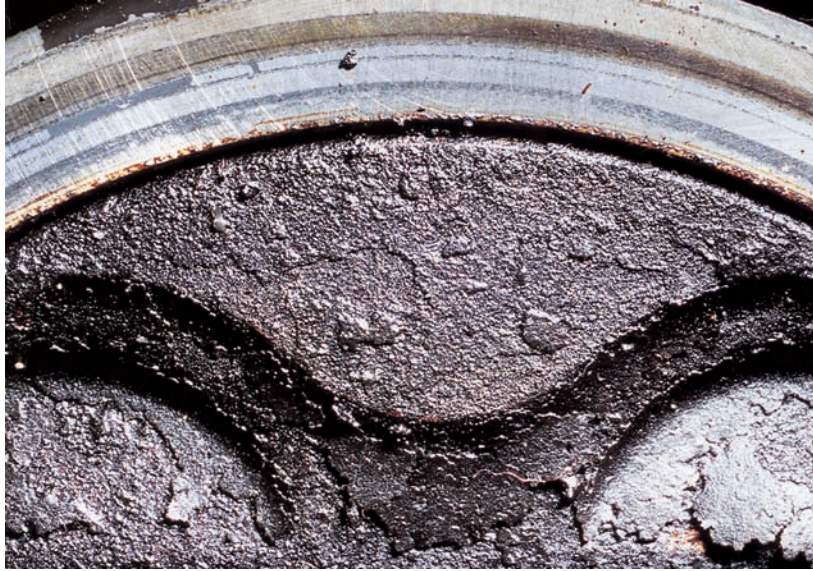
Combustion chamber squish area before.
