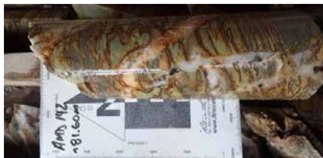
Figure 10: Foliation unconformable veining in hole AMD142 at approximately 81.6m downhole depth showing weak albite alteration with silica, ankerite, pyrite veins cross cutting foliation. (Willson, 2017)
