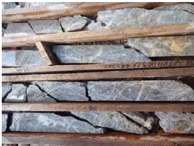
Figure 18: Typical silica, sericite, with biotite and albite quartz vein hydrothermal breccia showing near random vein orientations in hole TRD003 at approximately 99m depth down hole.
