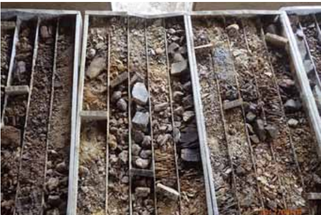
Figure 15: Section of SBD011 hole showing intense fault zone with flat/shallow foliation preserved.
