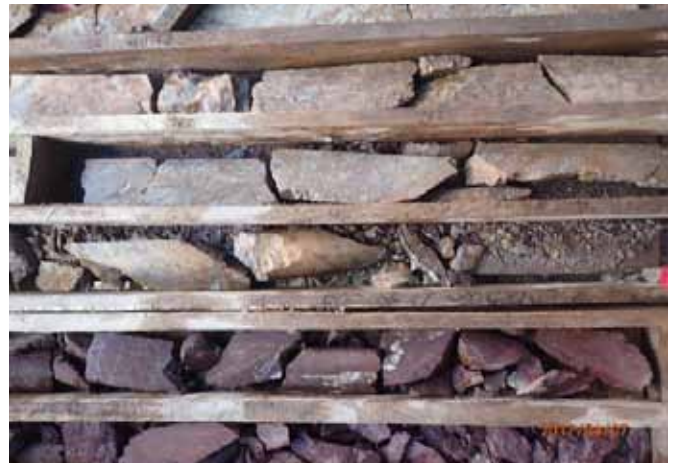
Figure 17: Sharp faulted contact between footwall hematitic mudstone and albite, silica, sericite altered hydrothermal breccia at approximately 92m downhole depth, TRD003.
