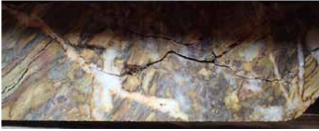
Figure 13: Image from AMD192 (depth unrecorded) within Lematik, showing early conformable veins (lower left), overprinted by unconformable veins (central left and right), cross cut by a disconformable breccia zone (central right).
