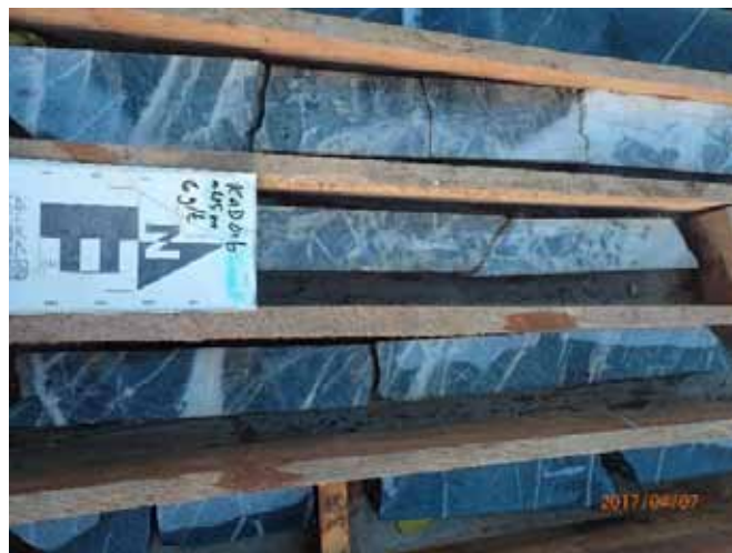
Figure 19: Mineralised intersection of KAD016 at the Kandeapi Prospect, Awak Mas project showing steep main vein with peripheral flat veins. Note proximal silica-sericite alteration.
