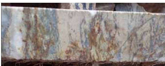
Figure 7: Core Photo – foliation conformable mineralisation from drill hole AMD142. (Approx. 65m downhole depth)
