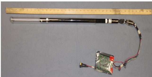
Fig. 5. The battery stick comprised of 8 individual Panasonic cells is shown along with the circuit board used for charging and discharging and safety. A meter stick is shown for reference.
