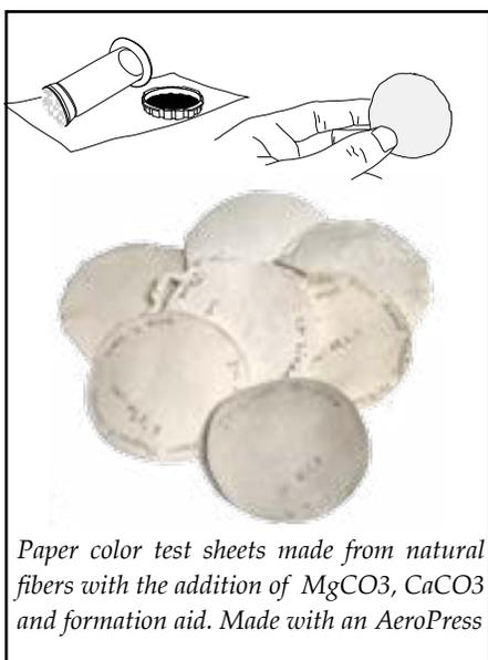
*Paper color test sheets made from natural fibers with the addition of MgCO<sub>3</sub>, CaCO<sub>3</sub> and formation aid. Made with an AeroPress*
