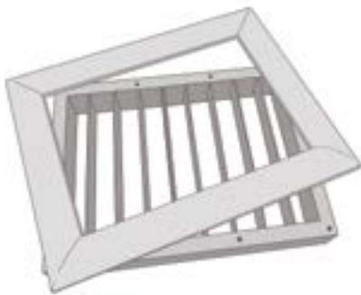
3-D printed traditional mould and deckle
