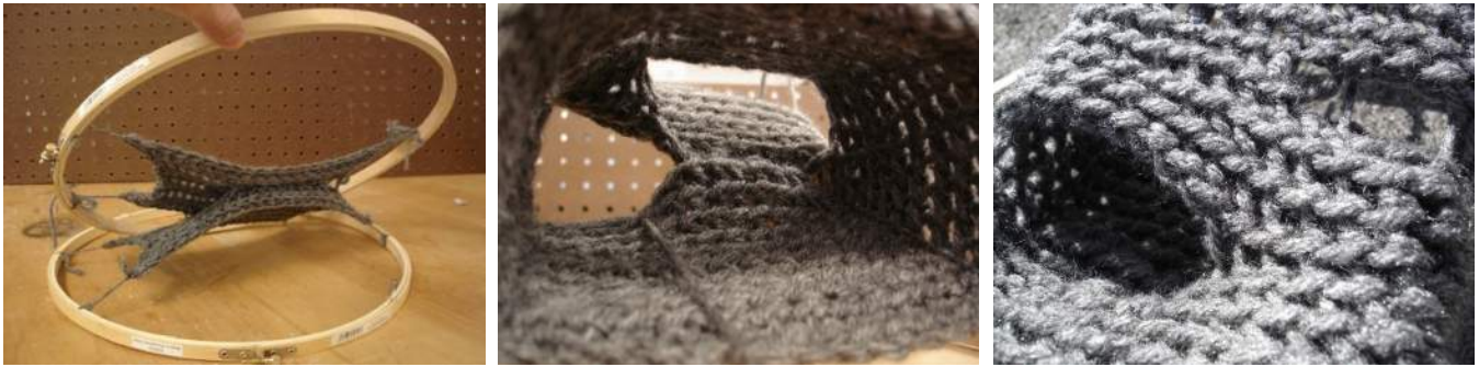
Figure 35-37: Analog experiments in creating new forms and spaces using a jig or formwork to engage the textile and enable the manipulation of the pliant model. In setting these rules, the textile model can be opened, closed, anchored, or stretched. The possibilities are only bound by the designer.
