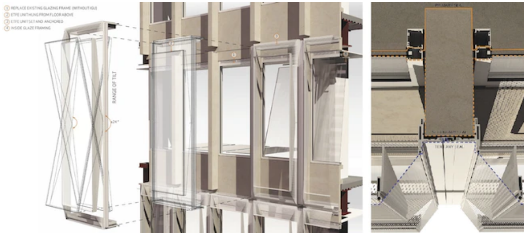
Figure 15 – Exploded assembly of Thermalswitch unit, Figure 15a – Plan view of precast batten with overlaid unit installed
