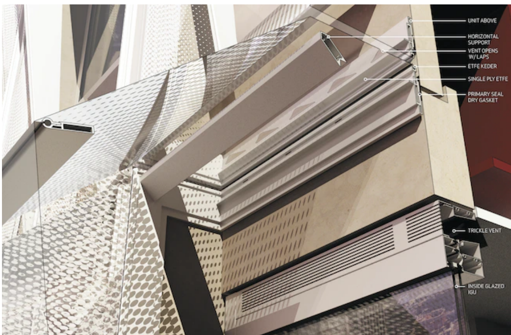
Figure 16 – Detailed rendering of Thermalswitch and punched window assembly with trickle vent
