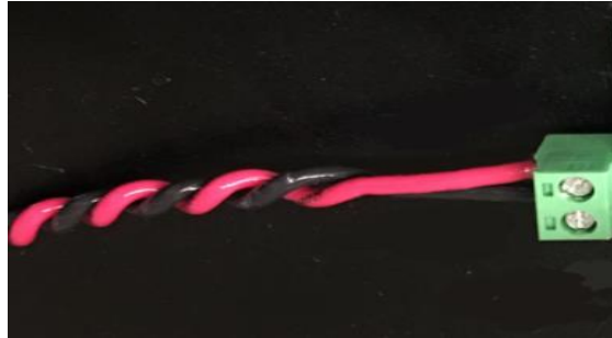
Figure 2: Example of Twisted Leads for Voltage Supply
