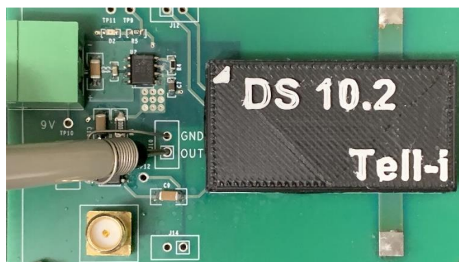
Figure 4: Example of Regular Probing Location
