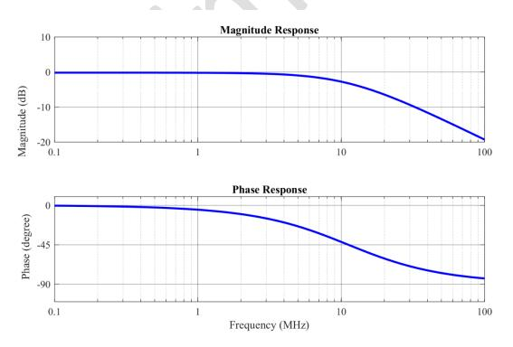
Figure 3. Frequency Response of Sensor (10MHz -3dB bandwidth)
