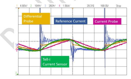
Figure 5 - Sensor operation in 1MHz switching converter with minimal inductor
