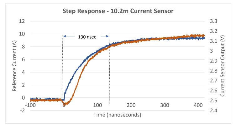
Figure 2. Step Response with 130 nanoseconds risetime.
