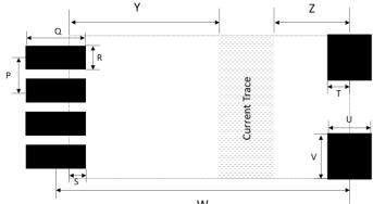
Figure 4. Recommended Hand Soldering PCB Footprint – DS50.2m The recommended Current Trace underneath – NO CONTACT- the sensor is 0.14" (3.56mm) wide.
