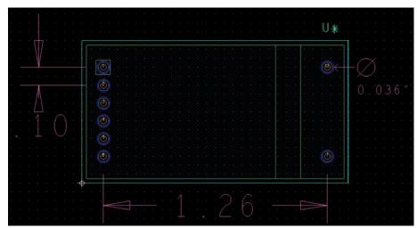
Figure 3. Recommended PCB Footprint, Grid Size:  $0.05'' \times 0.05'' - DS50.2$ . The recommended Current Trace width is 0.14''.
